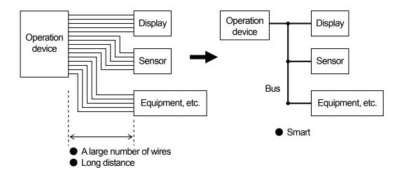
Historically, there have been a large number of wires for signal lines to connect equipment. By making the signals on these lines digital and putting them on a single cable, the number of wires decreases dramatically and it is much easier to maintain.
